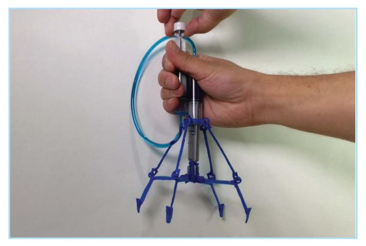
The Hydraulic Claw is made using two syringes and a length of rubber tube, the rest is 3Doodled!
