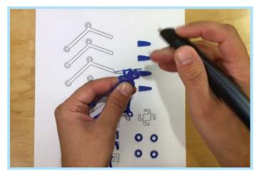
Doodle each side of the cross piece closed so that the fingers of the claw can dangle freely.
