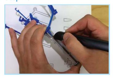
Attach the central cross piece the end of one of the plungers that you would normally be pushing on. Step 12
