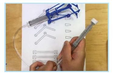
Attach the rubber tube to the tips of either syringe.
